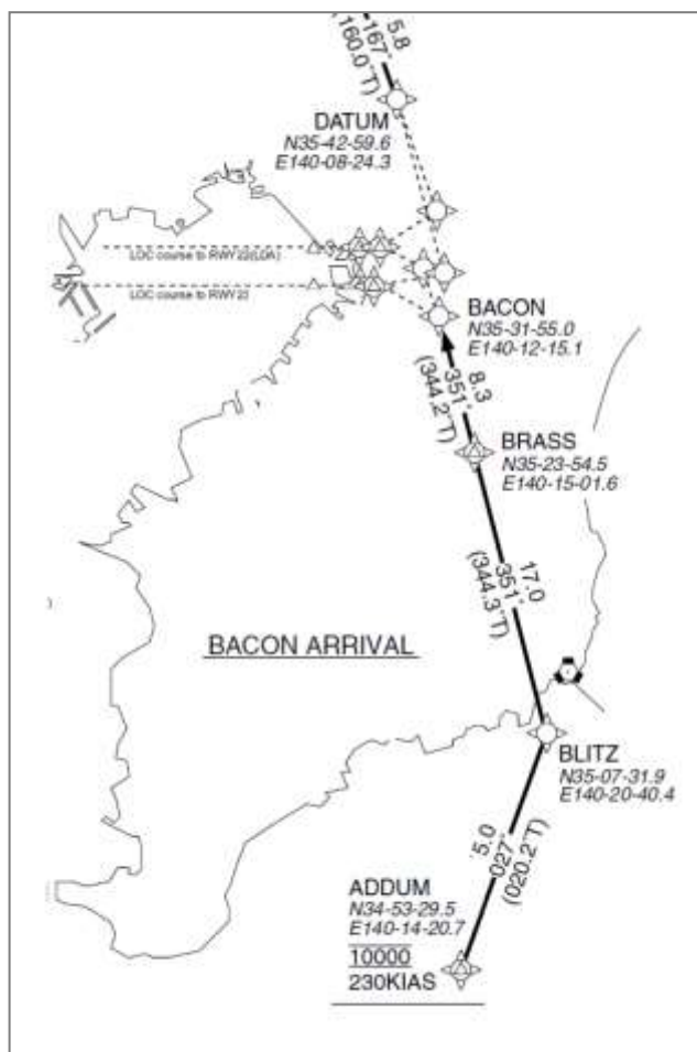
Figure 2 Example of the standard arrival course of Tokyo International Airport (RJTT) (RNAV STAR RWY22/23 BACON ARRIVAL) extracted from AIP-JAPAN
